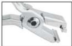
DE-1945 Detailing step pliers / Bayonet bending pliers - 1mm ● 0.30 mm to 0.50 mm (.012" to .020") ■ Max. 0.56 mm x 0.71 mm (.022" x .028")
